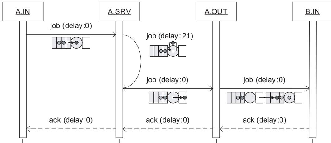
**Figure 3. UML sequence diagram of an example message flow. The  $(delay : D)$  labels indicate the elapsed simulation time before message delivery.**
